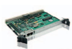
VM6050 6U VME Intel® Core™ i7 Single Board Computer
