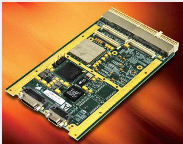
Sidebar Figure 2 | The SP0 3U CompactPCI SBC from Aitech is being used by various integrators working on NASA's Commercial Crew Vehicle program.
